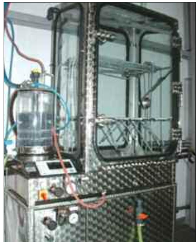
Environmental ageing chamber for ammonia atmosphere ageing
