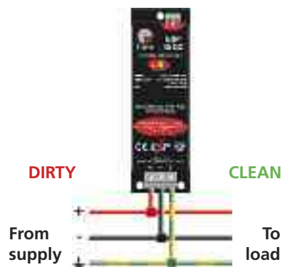
Parallel connection of ESP 48 DC
