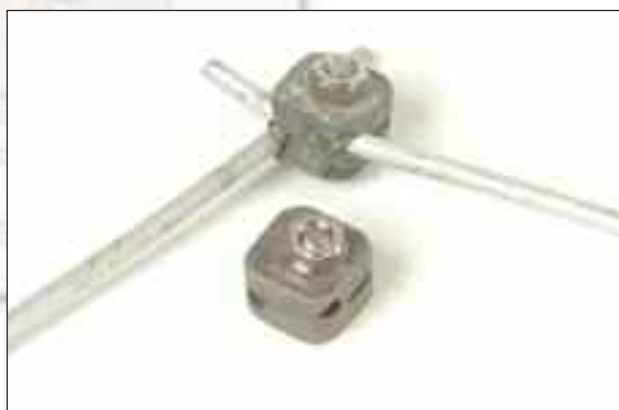
Furse lightning protection components, showing results after environmental preconditioning and lightning discharge testing
